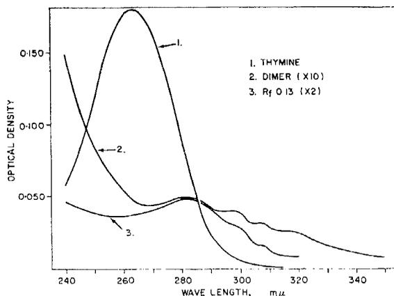
FIG. 3. Absorption spectra of thymine and its photoproducts
